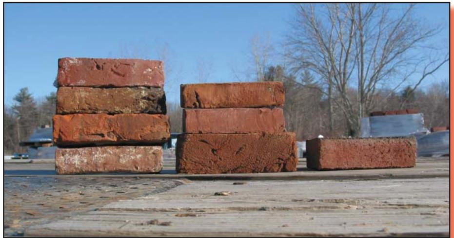
*Left to right: hand made 18<sup>th</sup> century brick, restoration brick, new wire cut brick.*
